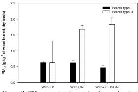
Figure 2.  $PM_{10}$  emission factors for the combustion in a pellet stove with or without passage of the flue gas through a pollution control device.
