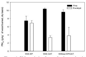
Figure 1.  $PM_{10}$  emission factors for the combustion in the woodstove with or without passage of the flue gas through a pollution control device.
